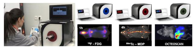
(Left) The  $\gamma$ -eye<sup>TM</sup> system in use, (Right) Top to bottom:  $\beta$ -eye<sup>TM</sup>,  $\gamma$ -eye<sup>TM</sup>,  $\varphi$ -eye<sup>TM</sup> systems, indicative images from the eyes with <sup>18</sup>F-FDG, <sup>99m</sup>Tc and Octeoscan respectively.
